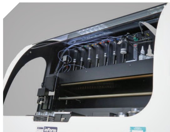
Pion's inForm machine allows us to precisely control pH monitoring, enabling dissolution studies under conditions that mimic in vivo conditions.
