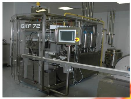
Our high-capacity Soft Gel production line is ready to serve with the latest technology here in Turkey by Vefa Pharmaceuticals. Gelatine is prepared in closed system and internal product is manufactured untouched by Soft Gel Encapsulating machine.
