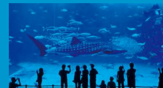
Large aquarium panel made of methyl methacrylate
