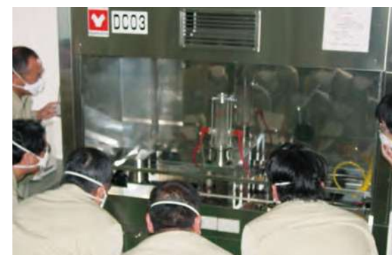
Dust explosion experiment conducted as part of training to acquire the ability to detect potential risks and respond appropriately
