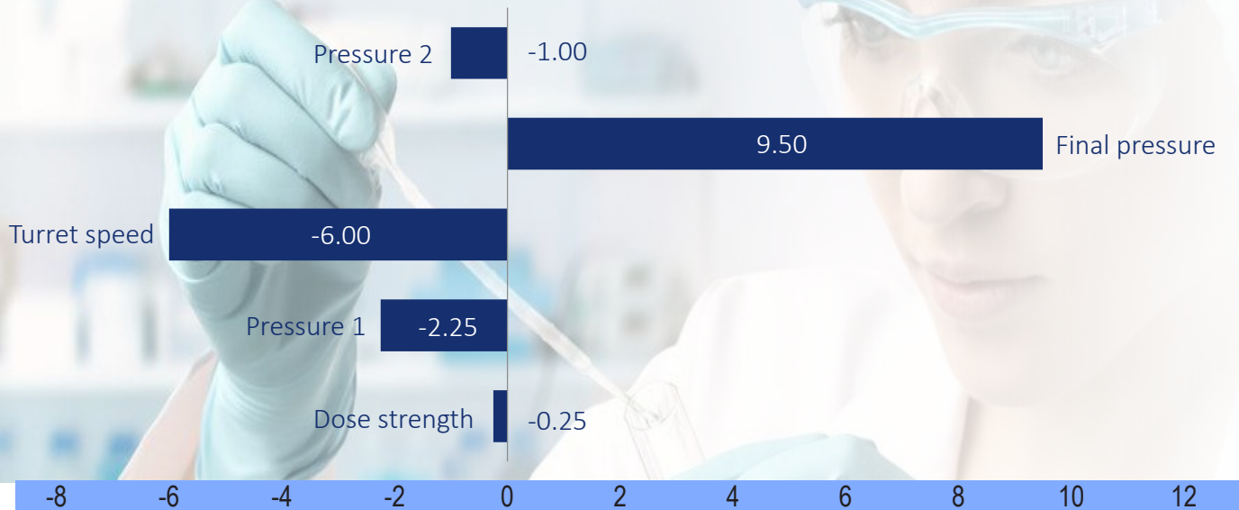
Case study: impact of 5 factors and their interactions on crushing strength
