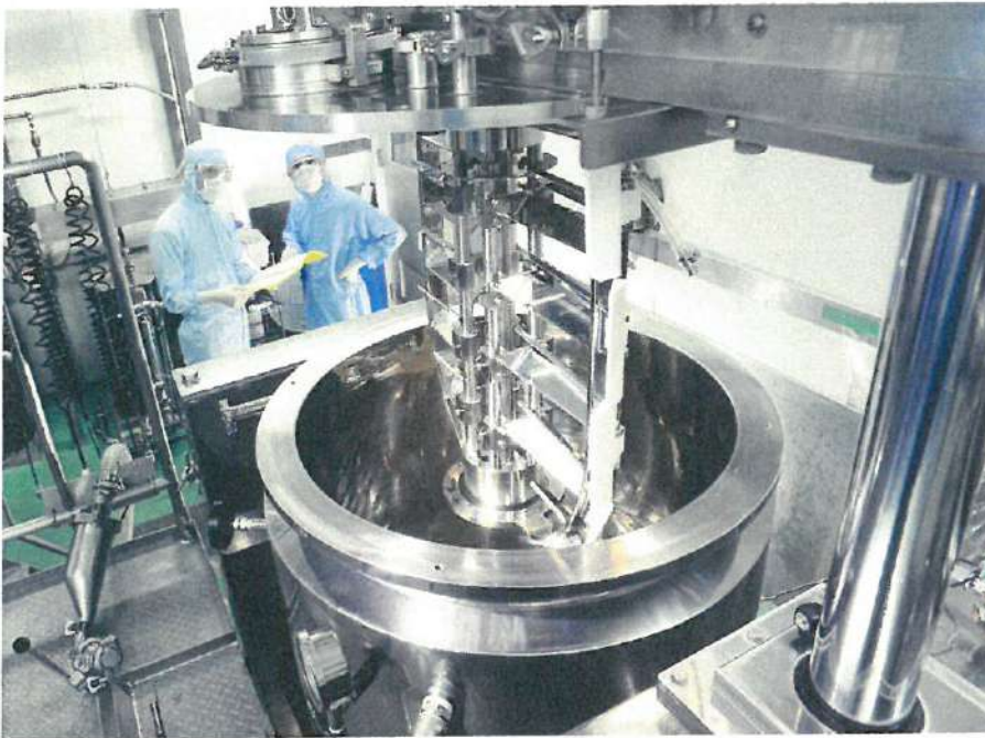
軟膏剤、クリーム剤の仕込みに欠かせない真空乳化装置 Vacuum emulsifying equipment essential in the preparation of ointments and creams
