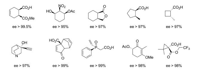
Chiral products obtained from PLE-mediated hydrolysis of carboxylic esters.
