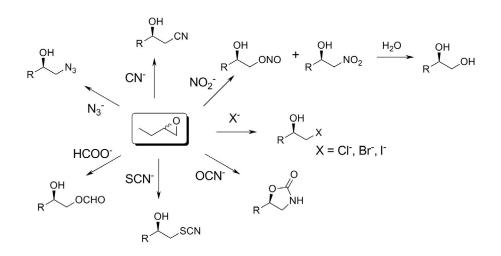
Catalytic scope of halohydrin dehalogenase-catalyzed epoxide-ring opening of 1,2-epoxybutane and various nucleophiles.
