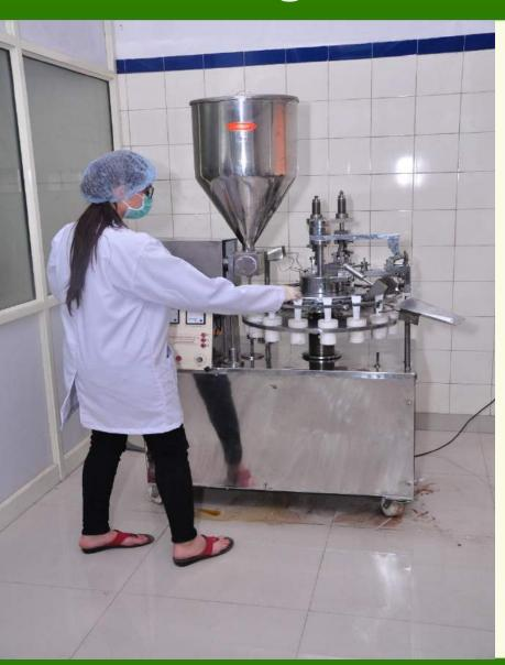
High capacity tube filling and sealing for releasing finished product for different testing and trial applications..
