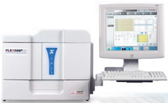
Figure 3.0 Flexmap 3D Luminex instrument, with xPONENT software Can multiplex up to 500 analytes
