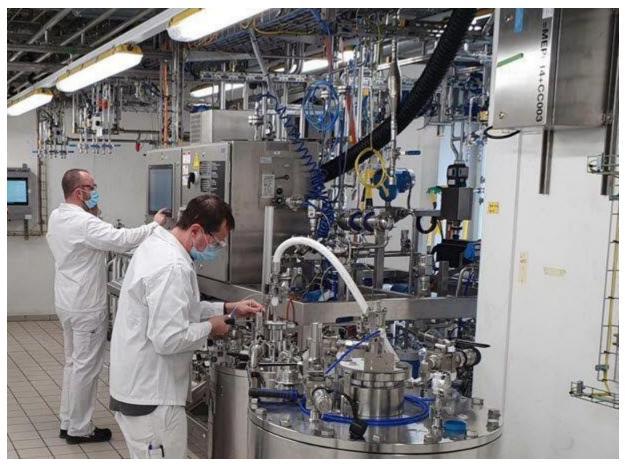
BACHEM'S LARGE-SCALE OLIGONUCLEOTIDE SYNTHESIZER
