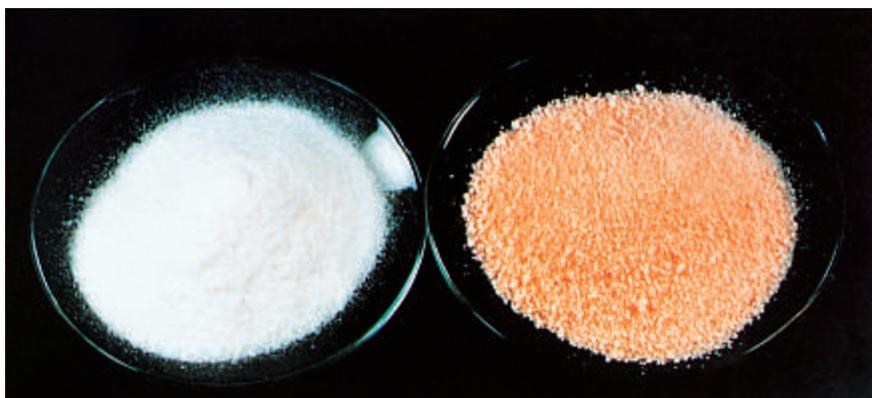
Fig. 2.40: Influence of different methods of wet granulation on the colour stability of ascorbic acid granulate with Kollidon® 30 (after 6 months at room temperature)
